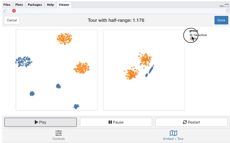
Figure 11: The clustering example from Figure 3 using the liminal interface. Here a grand tour is displayed on the right hand side, with buttons allowing users to play, pause and refresh the tour animation. Adapted from S. Lee et al., 2020, Figure 2.
